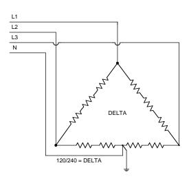
1.73 = )120V circuit voltage. This type of service can be found in industrial plants, commercial sites, and residential areas; the phase-to-phase voltages and phase-toneutral voltages are all commonly used for electrical circuits.
