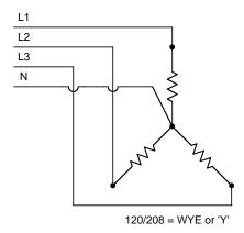
In a "Wye" power supply the hot legs of the 3-phase system are each connected to a grounded neutral. When diagrammed the circuit looks like the letter "Y" with each of the hot legs shown at one of the outer arms of the "Y" and the grounded neutral at the central junction point. The phase-to-neutral voltage is reduced by the 3-phase factor (Square Root of 3 = 1.73). E.g., for a phase-to-phase voltage of 208V, divide (208V by
