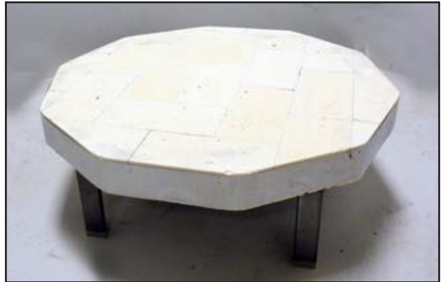
The kiln base positioned on the stand:
