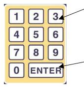
Numeric keys - Used for entering times, temperatures and other numbers. The number "1" is also used to acknowledge the ErrP error signal when you first turn the kiln on. Press "1", "2" or "3" while firing to change which thermocouple reading you see in the LED display. Press 8 while firing to turn On/Off the ability to see which zones are firing by the LED display dots.
