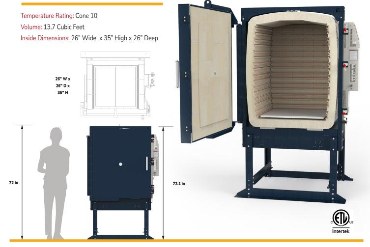
EFL Series Front-Loading kilns for studios and schools include arched sides and top for strength, heat-balanced insulation for even firing, adjustable door with plug seal, and door switch.
