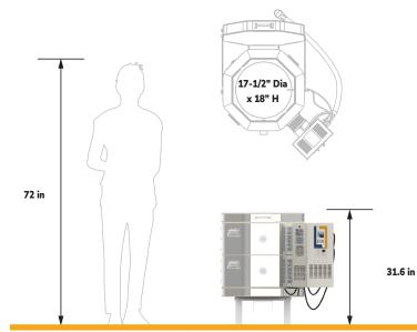
JH kilns are designed specifically for hightemperature crystalline glaze firing. Extra power, Quad element design, Type S thermocouples, and balanced super hightemperature brick for fast heat-up and fast cooldown make these kilns unique.
