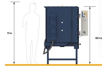
Commercial-grade front-loading kilns for production. Includes adjustable door with plug seal and fiberglass gasket, door elements, heavy-gauge welded case, 4.5" K25 arched brick top, door switch, and industrial control panel with branch fusing.
