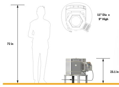
Small test and craft kilns that can run on 120 volts or low-amperage 208-240-volt circuits. These are great for beginning potters or for testing glazes.
