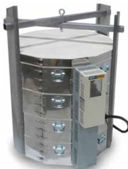
Heat-Treating Bell Kiln For Drill Bits
