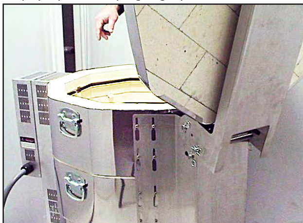
The properly Installed spring hinge open.
