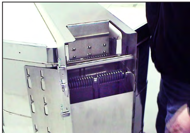
The properly Installed spring-hinge shown closed.
