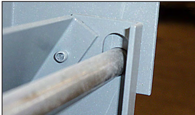
Positioning the hinge bracket.
