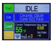
**Control:** Full digital touchscreen Genesis control with easy-to-use interface, WiFi enabled app, and simple programs for firing ceramics.
