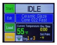
**Control:** Full digital touchscreen Genesis control with easy-to-use interface, WiFi enabled app, and simple programs for firing ceramics.
