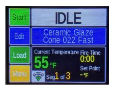
**Control:** Full digital touchscreen Genesis Mini control with easy-to-use interface, WiFi enabled app, and simple programs for firing ceramics or glass.
