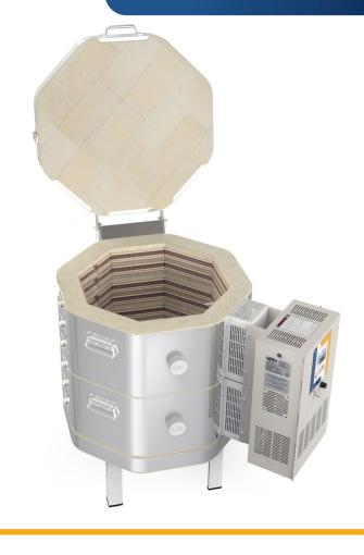
JH kilns are designed specifically for hightemperature crystalline glaze firing. Extra power, Quad element design, Type S thermocouples, and balanced super hightemperature brick for fast heat-up and fast cooldown make these kilns unique.
