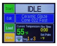
**Control:** Full digital touchscreen Genesis control with easy-to-use interface, WiFi enabled app, and simple programs for firing ceramics or glass.
