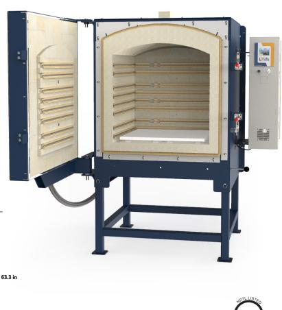
Commercial-grade front-loading kilns for production. Includes adjustable door with plug seal and fiberglass gasket, door elements, heavy-gauge welded case, 4.5" K25 arched brick top, door switch, and industrial control panel with branch fusing.
