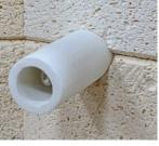
drop inside the tube where they can be vacuumed out during normal maintenance. (hotkilns.com/ protected-thermocouples)
