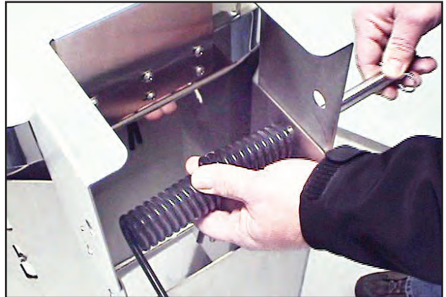
Installing the middle rod and springs.
