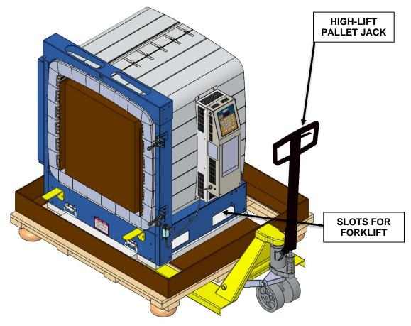
Once you lift the pallet with the high lift pallet jack or forklift, you will be able to drop the legs into the four cutouts in the cardboard and bolt to the kiln body using the provided bolts. Alternatively, there are slots in the sides of the frame you can use to lift if you have a forklift.
