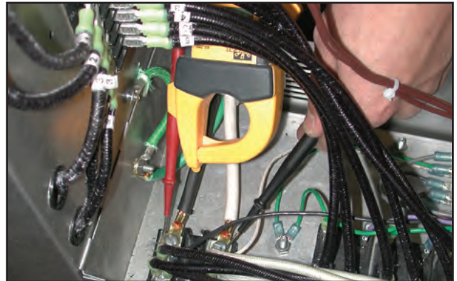
Checking voltage at the power terminal block.
