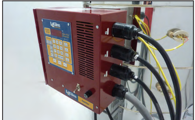
All element jumper cords installed:
