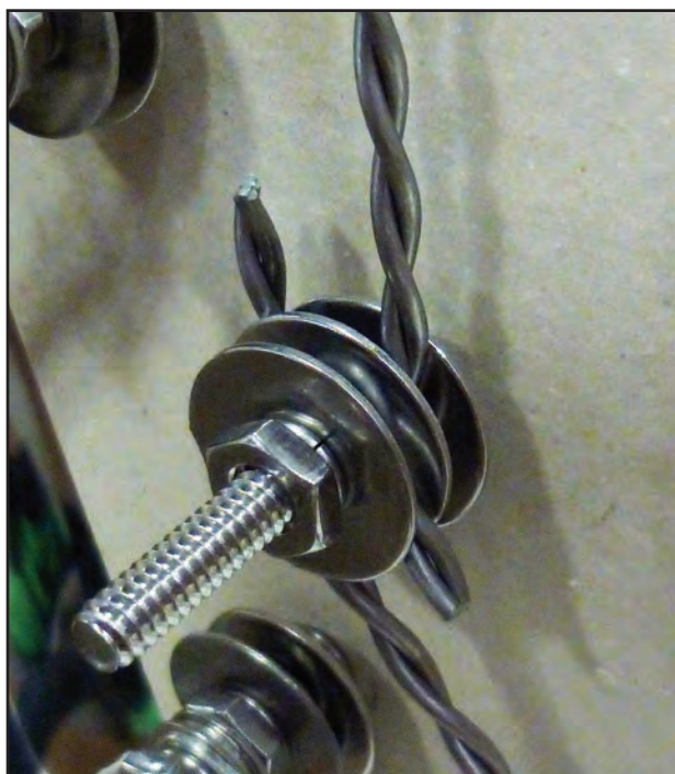
Detail showing how all the hardware gets assembled on the Terminal Bolt:
