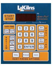
The time-tested DynaTrol with 4 Easy-Fire programs, 6 Vary-Fire programs, PreHeat, Delay, Program & Segment Review, and Diagnostics. Control is mounted on an angled panel for easy viewing. *Optional Genesis control (see page 8) features touch screen*
