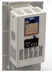
The panel is larger than the normal panel and comes disconnected from the kiln when packed. This must be reconnected in the field. (hotkilns. com/ssr)
