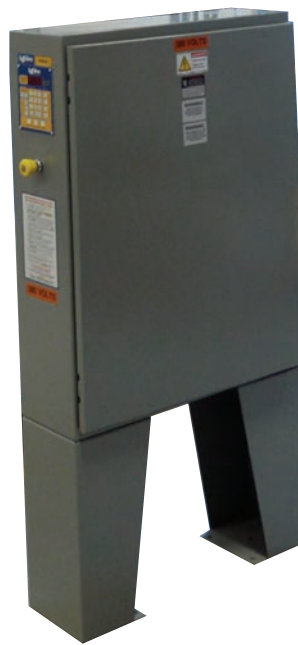
Kiln shown with the special control panel that houses the SSRs and/or High Limit Control
