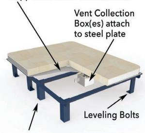
Welded heavy-gauge stand is powder-coated
