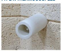
protects the delicate tip of the thermocouple from damage while loading. Also any metallic flakes from the thermocouple will tend to drop inside the tube where they can be vacuumed out during normal maintenance. (hotkilns.com/protected-thermocouples)
