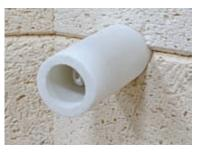
tip of the thermocouple from damage while loading. Also any metallic flakes from the thermocouple will tend to drop inside the tube where they can be vacuumed out during normal maintenance. (hotkilns.com/protected-thermocouples)
