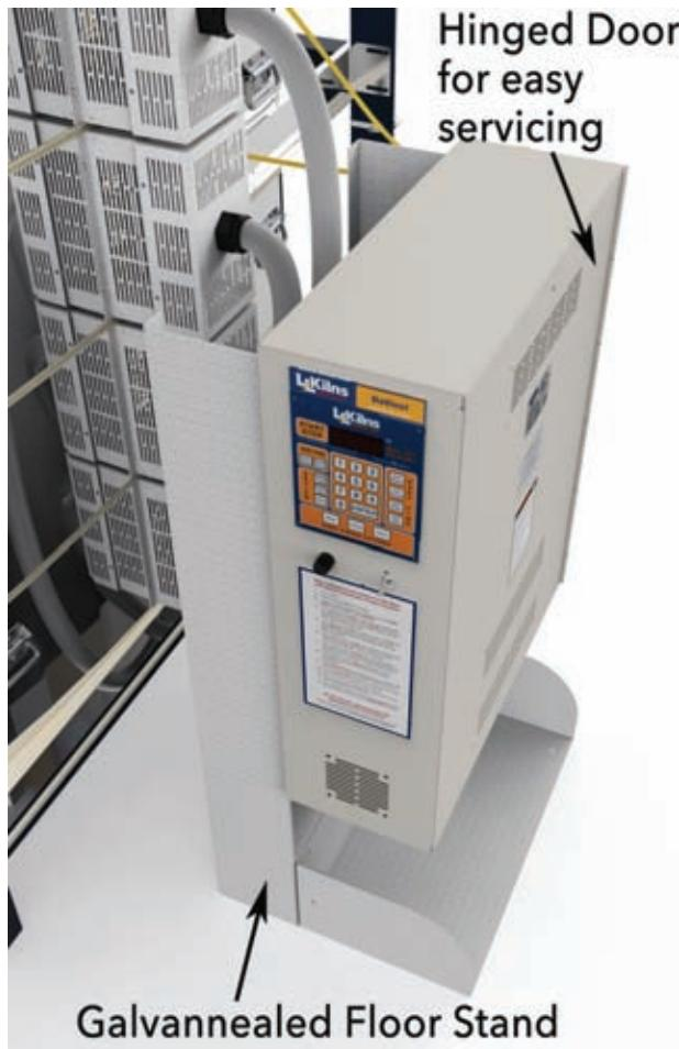
All controls and components are mounted in a separate control panel that floor mounted. Cords from the kiln sections plug into the panel. There is an air space between the panel and the kiln which keeps the controls cool - which is critical for long term health of the electronics. ([hotkilns.com/davinci-panel](http://hotkilns.com/davinci-panel))
