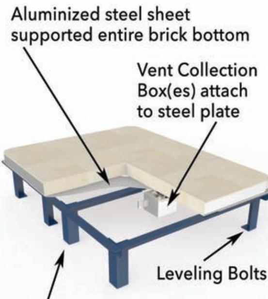
Welded heavy-gauge stand is powder-coated
