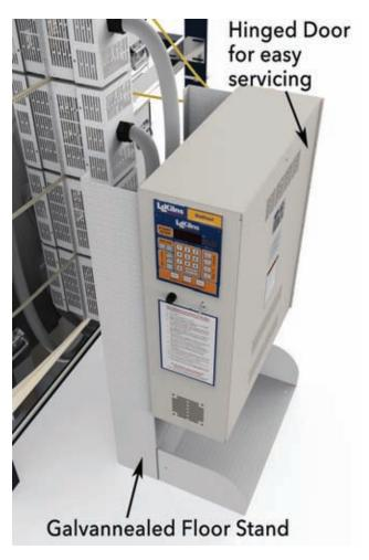
All controls and components are mounted in a separate control panel that floor mounted. Cords from the kiln sections plug into the panel. There is an air space between the panel and the kiln which keeps the controls cool - which is critical for long term health of the electronics. (hotkilns.com/davinci-panel)
