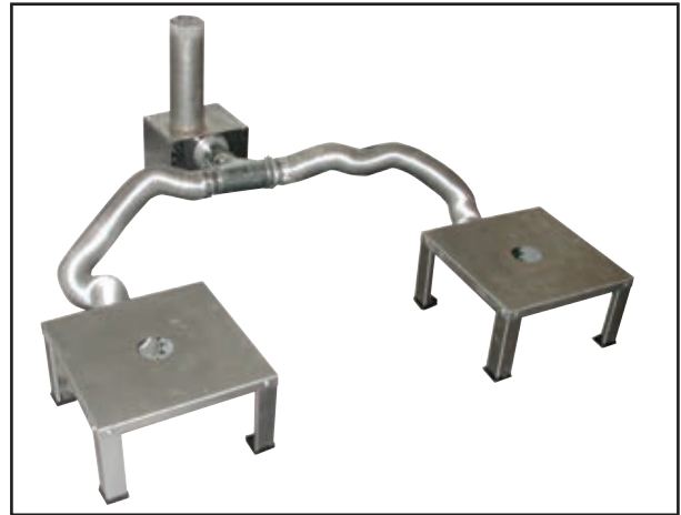
The Vent Doubler system includes an extra Bypass Collection Box, an extra Flexible Aluminum Duct and a "T" Connector with dampers. You can vent two 10 cubic kilns with one Vent-Sure plus this Vent Doubler System.
