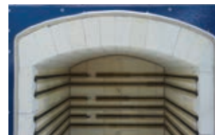
4-1/2" thick K25 Full Arch for extra strength
