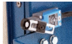
Safety Door Switch shuts off power when door is opened.
