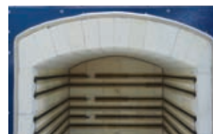
4-1/2" thick K25 Full Arch for extra strength
