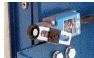
Safety Door Switch shuts off power when door is opened.
