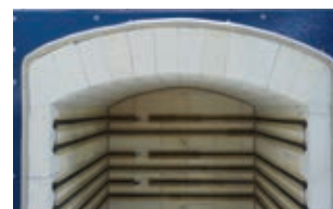
4-1/2" thick K25 Full Arch for extra strength
