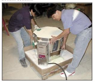
Place the kiln on the bottom slab and adjust it until the bottom section matches the bottom slab:
