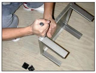
Fit the rubber-plastic feet over the bottom of the legs. The stand is now fully assembled:
