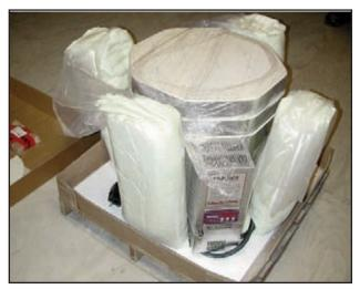
Cut off the foam pads with a box knife:
