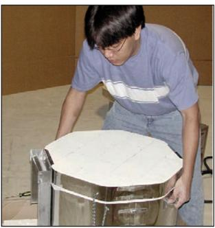
NOTE: Usually the top section along with the top is light enough that you can move it as an assembly. However, if you need to remove the top you can remove the screws that hold the support chains to the kiln and remove the hinge bar. Again - be careful of lifting too much weight.
