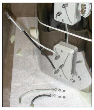
Now that the two sections are disconnected from each other you can lift up the top section. Place it down on the ground temporarily:
