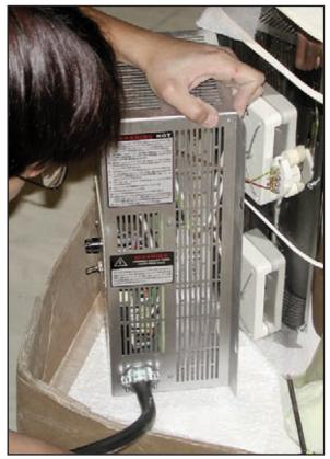
Unscrew the thermocouple wires. Notice that the red wire goes next to the thermocouple wire that is marked red.
