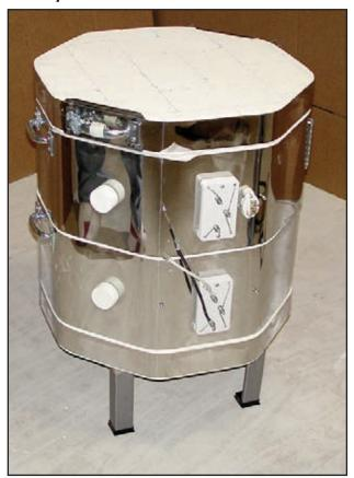
Reattach the Element Jumper Wires that go between the sections and attach the Element Connection Wires:
