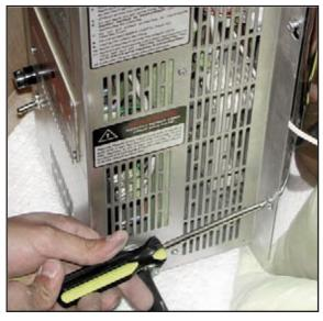
Lift the panel up slightly to slip it off the two screws on the right. Let the panel hinge to the left by leaving it loosely attached to the left screws.
