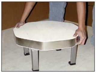
NOTE: Level the kiln. Do this before proceeding because at this point it is easy to put a level on the flat bottom. Use metal shims under the legs to accomplish the leveling. We suggest using a carpenter's level for this job. Make sure that the base will not wobble.
