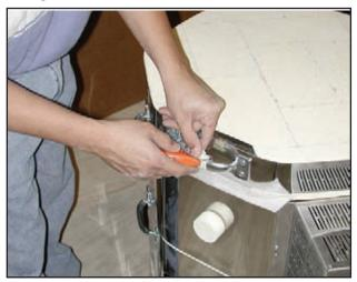
Install the hook into a wall so you can attach the safety chain when the door is up: The kiln is now fully assembled and ready to plug in to a 30 amp circuit and operate:
