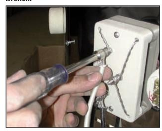
Leave the Element Jumper Wires attached to the bottom section - just remove them from the top:
