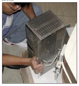
Reconnect the thermocouple wire. BE SURE TO CONNECT THE RED WIRE TO TERMINAL THAT HAS THE RED MARK ON THE WIRE STUB PROTRUDING FROM THE THERMOCOUPLE:
