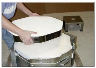
Place the bottom of the kiln on the kiln stand. Center the bottom brick on the stand. It is not critical how the polygonal brick is oriented to the square stand:
