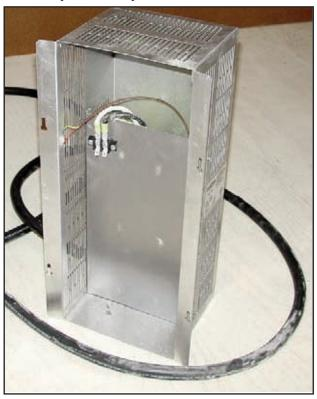
Remove the terminal nuts on the top element terminal block so you can remove the element jumper wires that go between the two sections. Use a 3/8" nut driver or socket wrench:
