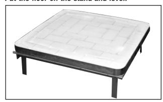
LEVEL THE KILN! This is important because the Dawson Kiln Sitter is affected by gravity. If the kiln is not properly leveled the Kiln Sitter might be either too reactive or too sluggish. ALSO IF KILN IS NOT LEVELED THIS COULD LEAD TO THE CRACKING OF THE BOTTOM AND THE TOP
