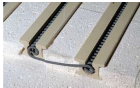
Detail showing the top with hard ceramic element holders that prevent most dusting of the soft firebrick
