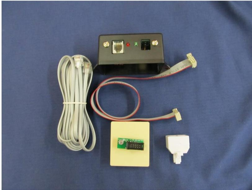
Once the computer portion of the installation has been completed, you are ready to install the hardware on the kiln and connect each kiln to the system. Above is a picture of the Kiln Kit that will be used on each kiln installed
