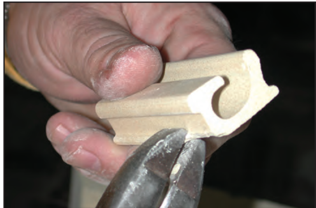
Using Linemen's Pliers snap off the BOTTOM edge of the holder
