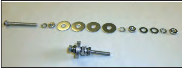
Detail showing how all the hardware gets assembled on the Terminal Bolt:
