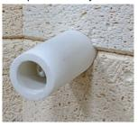
from the thermocouple will tend to drop inside the tube where they can be vacuumed out during normal maintenance. (hotkilns.com/protectedthermocouples)
