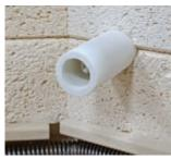
from the thermocouple will tend to drop inside the tube where they can be vacuumed out during normal maintenance. (hotkilns.com/protectedthermocouples)
