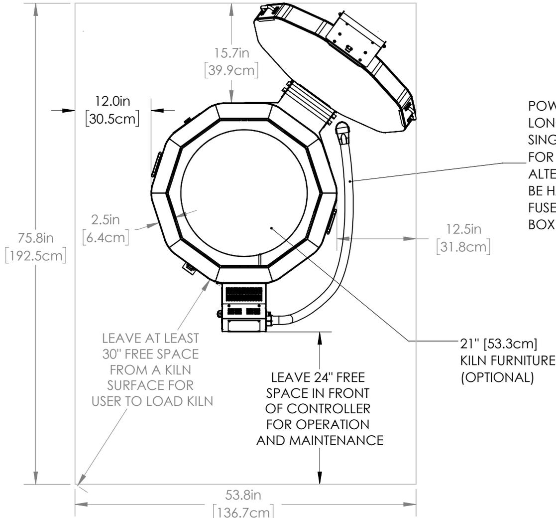
POWER CORD IS 6 FEET LONG: NEMA 6-50 FOR SINGLE PHASE OR 15-50 FOR THREE PHASE. ALTERNATELY KILN MAY BE HARD WIRED TO A FUSED DISCONNECT BOX.
