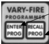
**ENTER PROG** - This button allows you to initiate programming. Up to 6 profiles (programs) may be programmed and saved.
