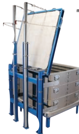
This shows the spring hinge system in the back
