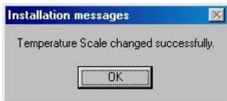
If the user selects a change in temperature scale, the watch icon will be displayed. This indicates the message to change the temperature scale is being sent and KISS is verifying that the controller received the message correctly and the scale did get changed. When all that is finished, the above message indicating the temperature change has occurred.
