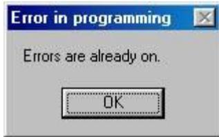
This error message is displayed when the user has selected to turn on the error checking feature, but the feature is already on at the controller.
