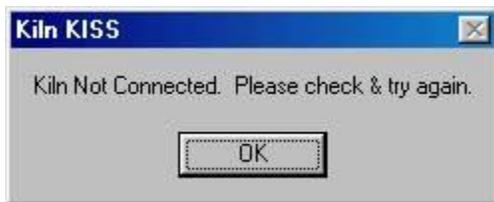
This error message is displayed when the user has selected to start the kiln, the controller is responding to the message from KISS, but is continuing to indicate a status other than "Firing". One possible explanation for this situation is a user stopping the firing at the keypad in between when KISS sends the message to start the kiln and when the controller answers back to KISS when it tries to verify that the kiln actually started.
