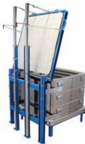
Spring-loaded Counterbalanced Lid
